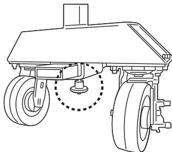
3. Tighten the knurled adjustment bolt that secures each outrigger base assembly to the tie bar to dollies bearing the full battery weight. **NOTE: Failure to tighten adjustment bolts prior to the dollies bearing the battery weight may result in unsafe shifting/detaching of the outrigger base assembly.**
