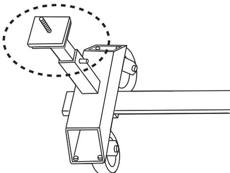
1. Set the height adjustment for all four extension pad assemblies to the desired height.
