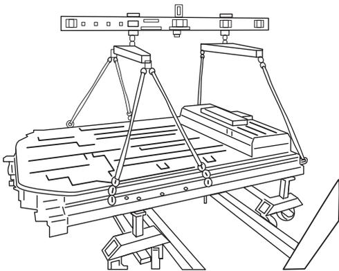
2. Use an approved lifting apparatus to suspend the battery in the correct position over the dollies. Slowly lower the battery onto the dollies while adjusting position as necessary.
