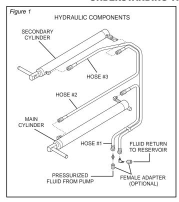
Many systems require flow dividers, flow control valves or load equalizers to guarantee that both lift pads raise the vehicle relatively level. The model 86006 eliminates the need for a load equalizing device by using double acting cylinders equipped with internal bypass valving. Refer to figure 1 for identification of hydraulic components and an explanation of the system.
